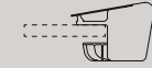
External top access Top access esterno L 40 cm, W 23 cm, H 17 cm L 15 ¾", W 9", H 6 ¾"
